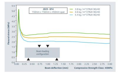
Note: These curves are based on averages of several beam tests. The toughness performance will depend on the concrete mix design used.
