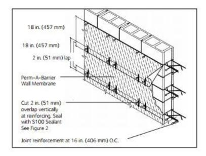
For PERM-A-BARRIER®High Temperature Wall Membrane, secure top edge of membrane with mechanical termination bar fastened securely into the structure.
